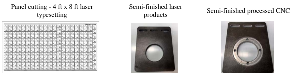
Figure 3 Schematic Diagram of Panel Cutting and Motor Bearing Semi-Products
